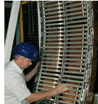
High-power ELM-resistant RF antenna
